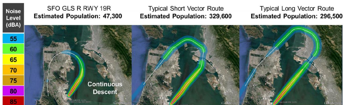
Figure 16: Comparison of noise exposure in San Francisco between a RNP approach and two kinds of radar vectors.
